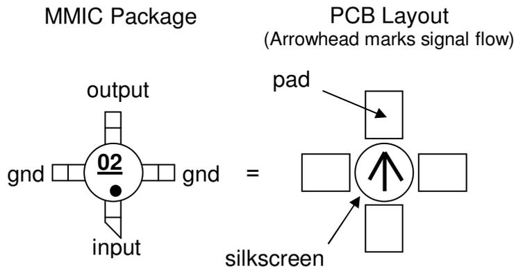
**Fig 2** MMIC physical appearance and corresponding PCB layout
