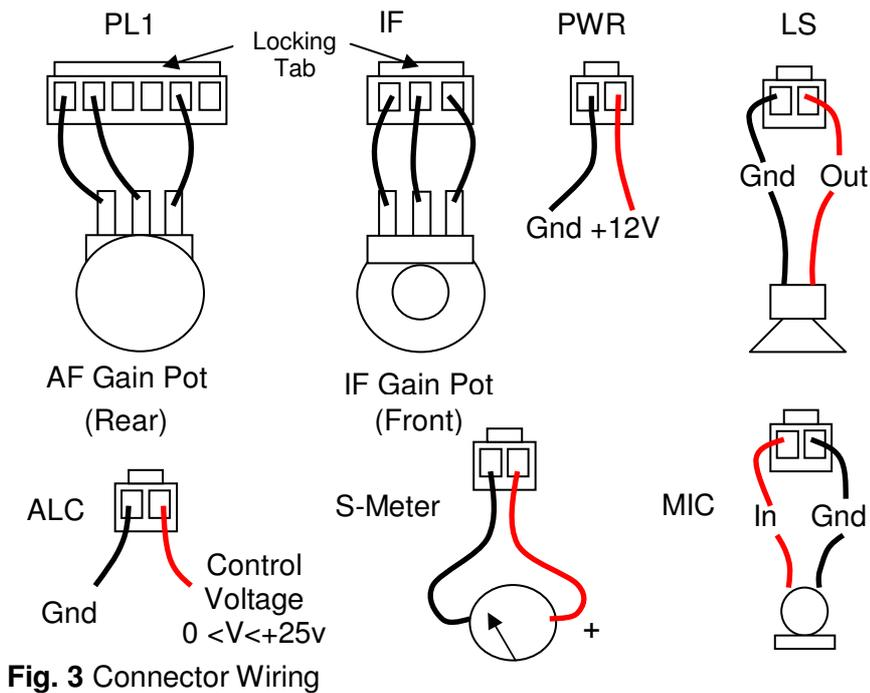
**Fig. 3** Connector Wiring
