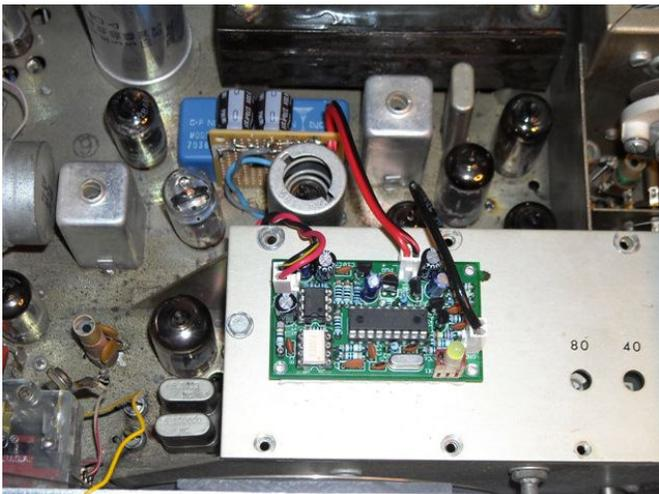
**X-Lock mounted on VFO Cover, Figure 4**
