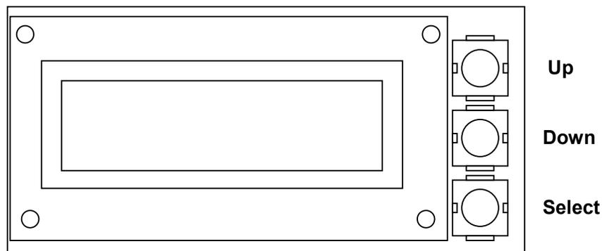
Fig.6 Button functions in "Set Up" mode
