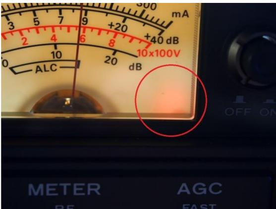
Fig 6. X-lock after slight VFO movement to allow the Red LED to be seen.
