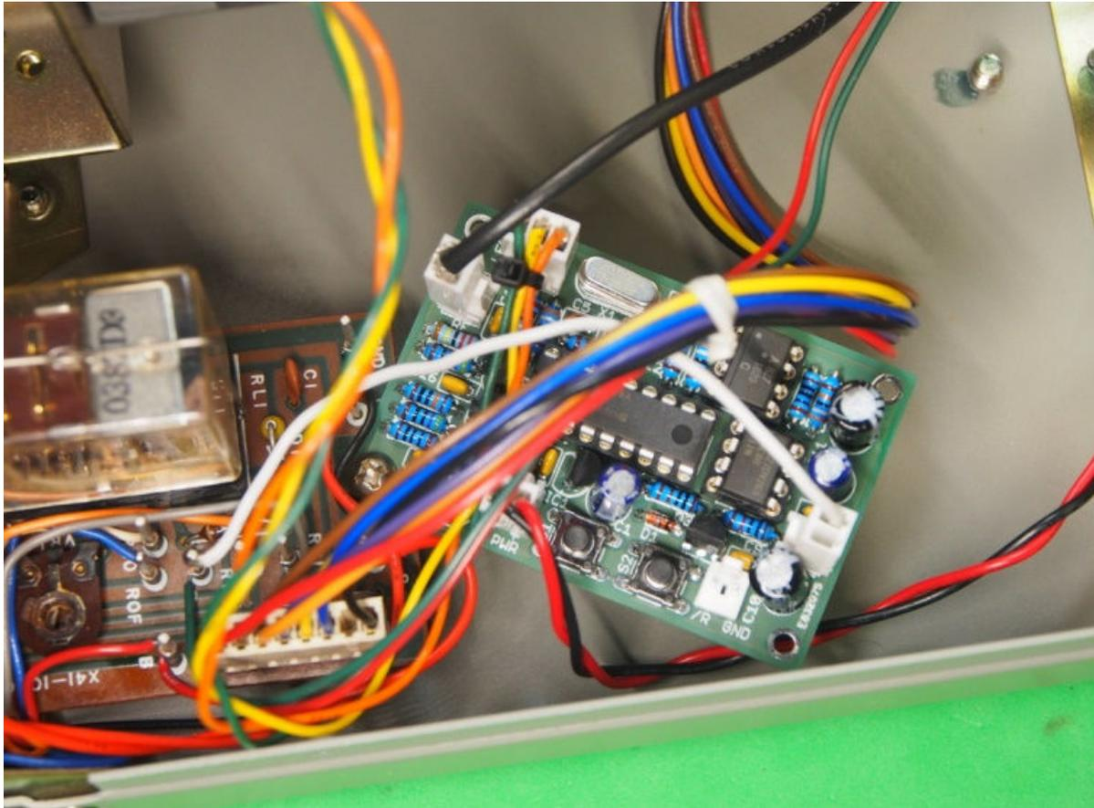
Fig. 2 X-Lock mounted to native circuit board with connections.
