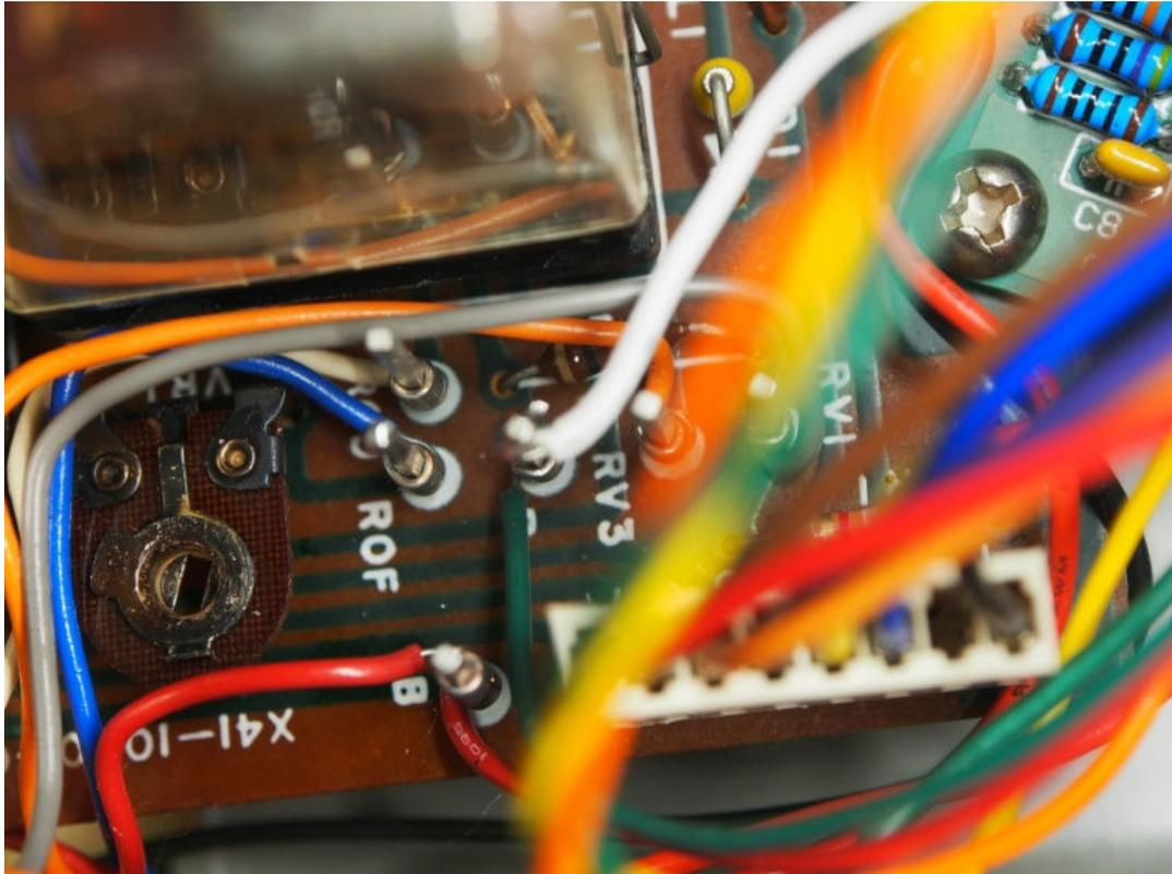
Fig. 3 White wire from VAR output of X-Lock to RV3 pin of the native VFO circuit board. VR1 also seen in this picture for adjustment of the RIT after installation.
