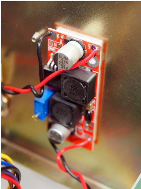
Fig. 1 DC-DC step-up module on back panel.
